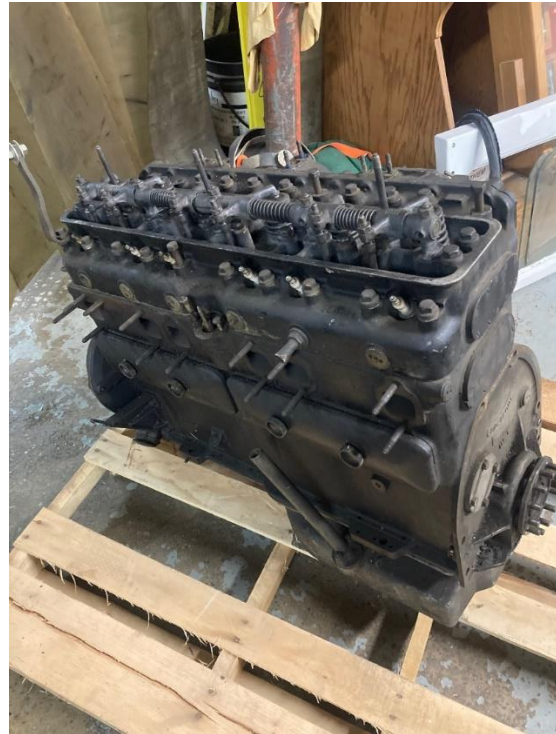
Bentley flat head 6 cyl. "oise" engine
